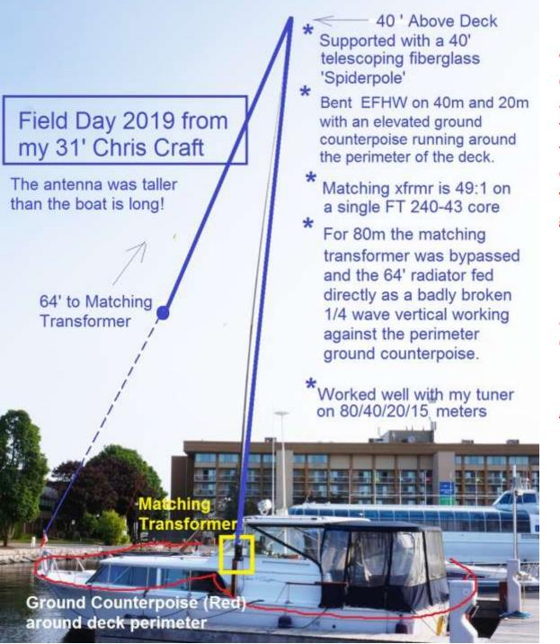
Another variation that I came up with while wintering in Florida, configured so that I could connect a ½ wave radiator to the matching transformer, or I could bypass the transformer and feed the radiating element directly and work it as a vertical antenna against a raised ground counterpoise.
