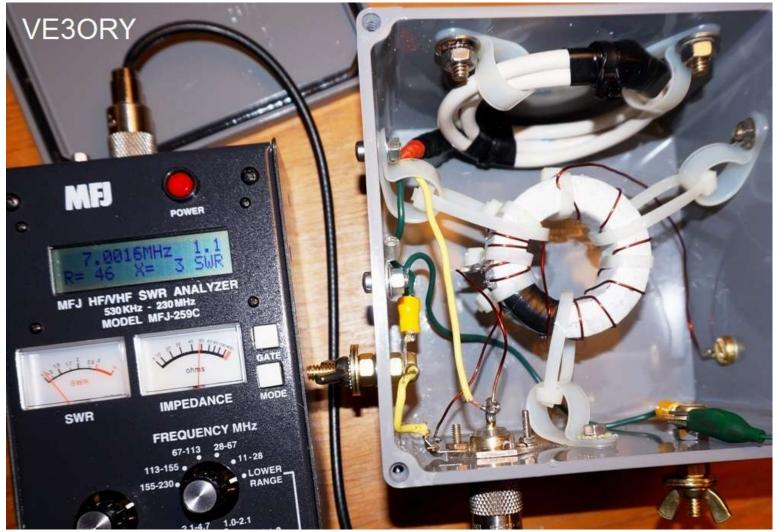
Here is a plot of SWR for one of my transformers taken using an MFJ-259C antenna analyzer. Fairly pleased with this one, as the SWR is less than 2:1 across most of the HF band. I have found it relatively easy to obtain good results when winding on a single core. It seems to become more difficult when stacking multiple cores for purposes of better power capability. I think in theory due to resulting higher inductances.
