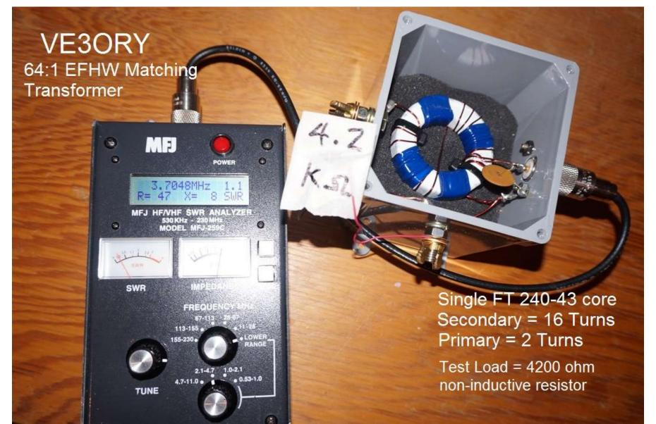
For this transformer I experimented with using a piece of coax cable to provide the capacitance across the input winding. You can do without this capacitor if your antenna is targeted for the lower bands (80/40m) and you don't care so much about SWR increasing at the higher frequencies.
